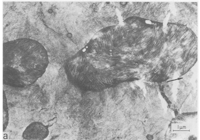
Figure 10 Transmission electron micrographs of modified PP (stained). (a) CO/HDPE (b) PP/PE-copolymer
